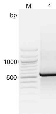
Agarose gel (1.5%) analysis of 1 µl transcription product in 5 µl loading buffer (M: Marker; Lane 1: 480-bp dsRNA) produced by esiSCRIBE with the reference template.
